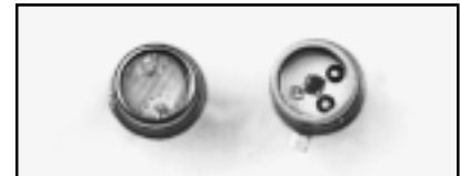
Figure A.3. Typical photocell (left) and phototransistor (right).
