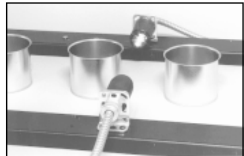
Figure A.1. Early photoelectric sensors used an incandescent bulb light source.
